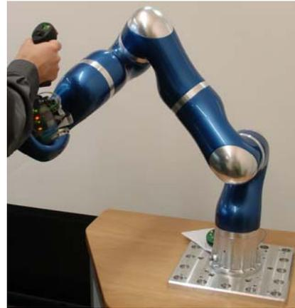
Figure 4: Robot arm for tele-presence control
